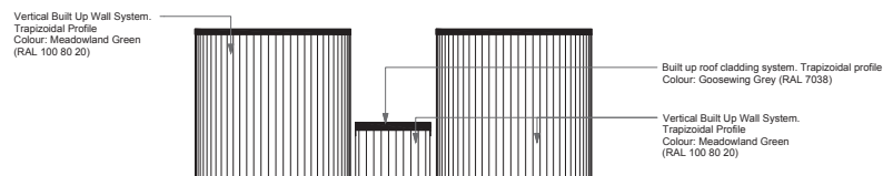
Sprinkler Tanks and Pump House Elevation E
