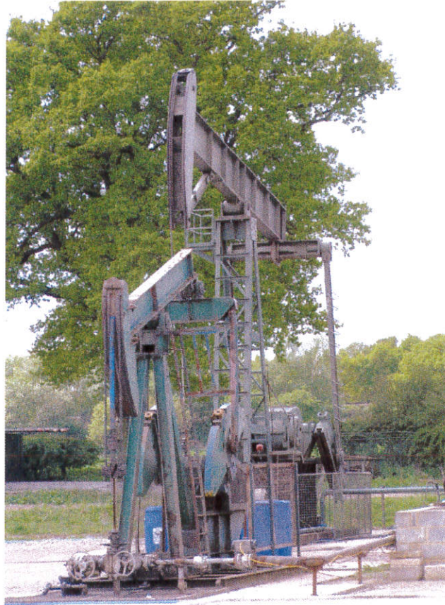
The two 'nodding donkey' beam pumps at Brockham.
