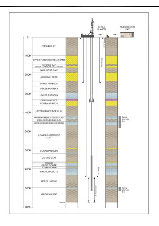
Notes: A 15/08/13 Amended well diagram EC LW Ckd By Rev Date Description Hydrock 113 4th Floor, Churchill House Regent Road Hanley Stoke on Trent ST1 3JJ TEL: 01782 261 919 FAX: 01782 262 020 E-Malt: stoke@hydrock.com or visit www.hydrock.com CELTIQUE ENERGIE PROPOSED HYDROCARBON **EXPLORATORY BOREHOLE** (WISBOROUGH GREEN #1) Figure 11.5: Borehole Diagram FINAL C/13054 Checked Scale at A3 Date Issue Date LW EC NTS | 22/03/13 | 22/03/13 C13054/02/005 Α
