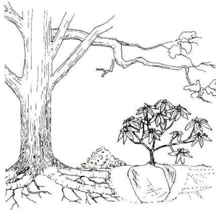
Root severance as a result of planting within RPA
