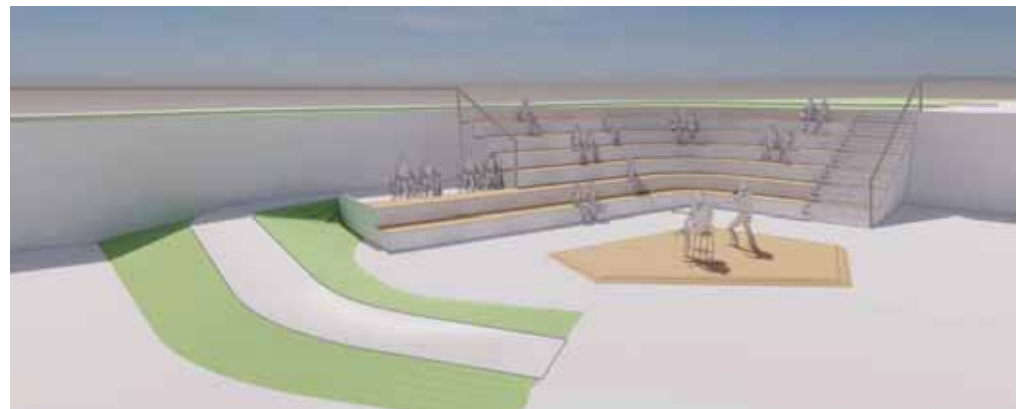
Sketch design of amphitheatre with wheelchair platform and 1 in 21 slope ramp. Performance area in centre for variety of uses.
