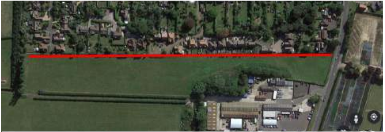
Figure 3 - Temporary Noise Barrier Location Along Eastern Boundary of Site
