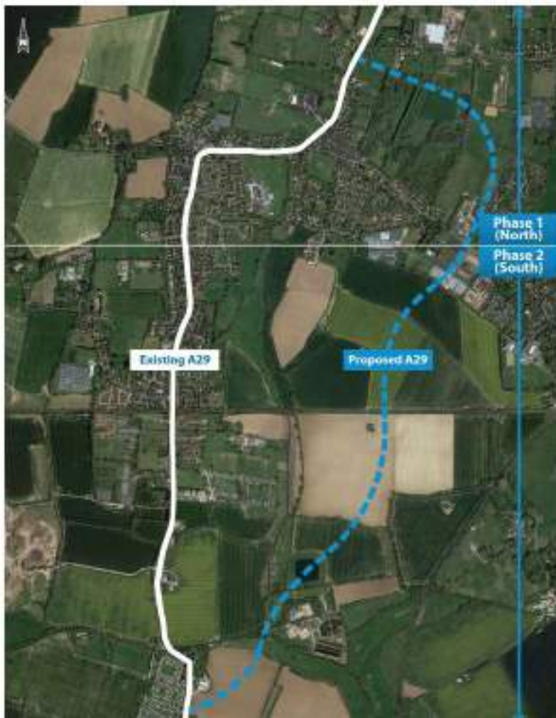
Figure 2 A29 Realignment Phases
