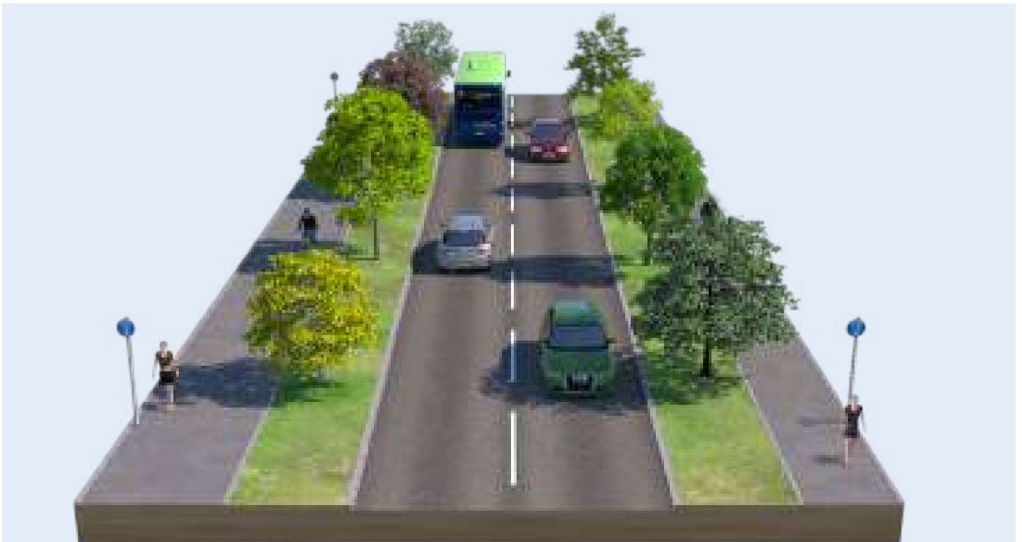
Typical example of cycleway/footway with green verges
