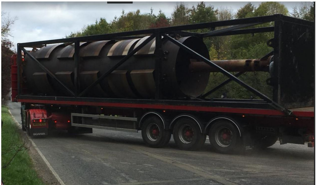
Flare stack (that burns off unwanted gases – and produces NOX) leaves.
