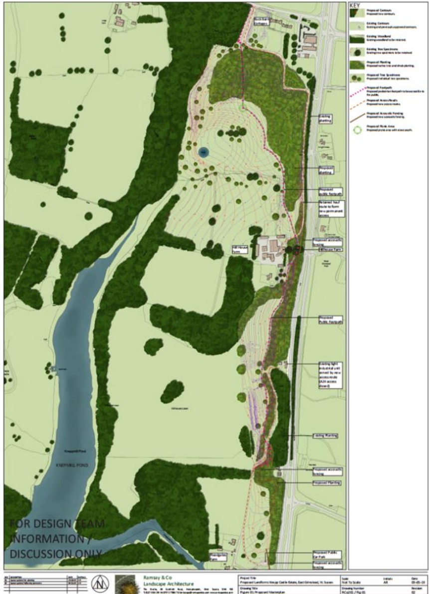
Fig 6 plan of the proposal to extend the new earthworks from Buck Barn Field to Hill House Farm and on to Floodgate Farm
