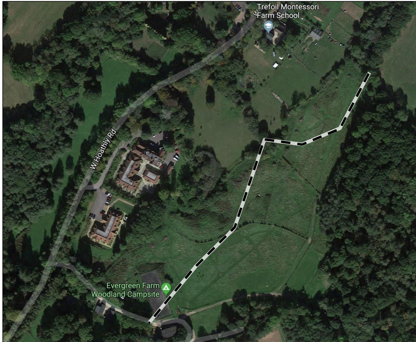
Figure C-3 – Approx. 110 m distance line for works beyond which guideline noise limits are met for long-term works
