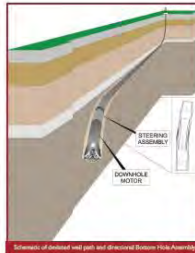
Schematic of deviated well path and Directional Bottom Hole Assembly
