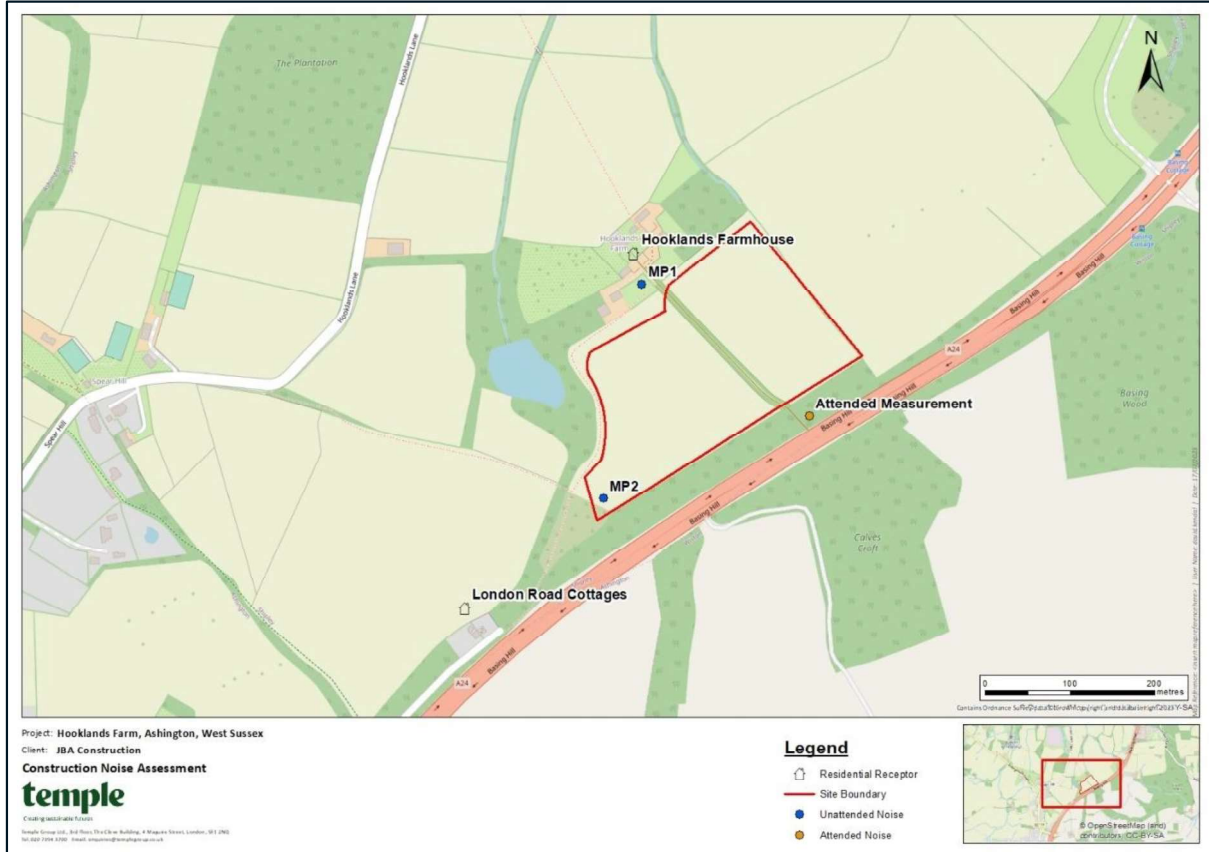
Figure 1 Survey measurement locations
