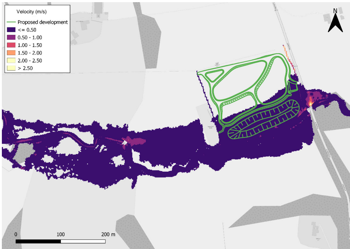
Figure 3.5: Modelled water velocities in the 1% AEP plus climate change event baseline scenario
