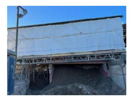
The trommel is around 11.5m long – the height of the structure is approx. 3m, with an overall height of 7m (above ground level)
